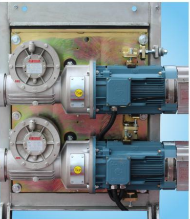
国产电机二传动 Two-motor for domestic drive.
